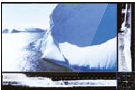
Style 2. Horizontal and vertical waveform with small vectorscope
