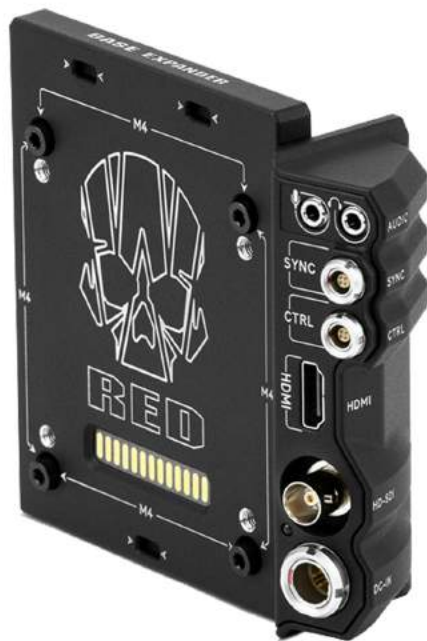
Figure: DSMC2 Base Expander
